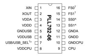
Note: ^: Internal pull-up resistor
